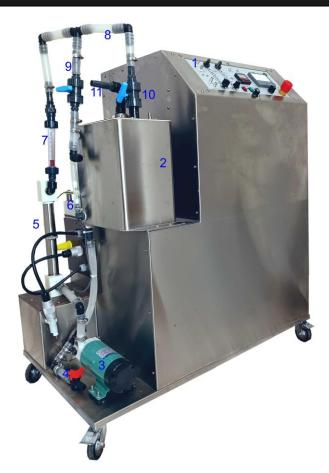
• **coaxial PEF chamber** for liquids with three replaceable central electrodes for 3-, 4- and 5-mm gaps to the wall.
